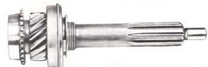
Connects the clutch plate to the input shaft of the gearbox. The splines on the input shaft locate into the clutch plate centre hub, where engine torque is transferred to the helical gear of the input shaft, this helical gear is in constant mesh with the gears on the lay shaft
