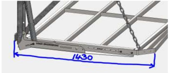
1. Measure the distances from the face of both posts to the platform. These measurements should be within 20mm of each other and less than or equal to 1490mm. If not, spacers may be required to make both sides the same.
