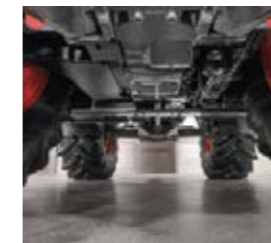
■ True ground clearance of up to 50 cm – no low parts such as stops or cables
