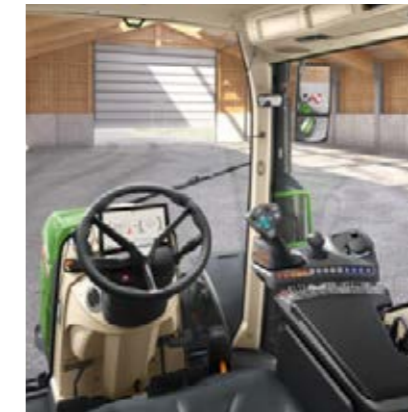
Profi Setting 1 - Crossgate lever - 1 linear module (rocker pair) to control hydraulic valves
