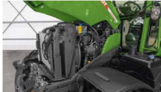
The engine compartment is very easily accessible for inspection and maintenance, even with front loader attachments. The bonnet has two separate side parts to make it easy to open.
