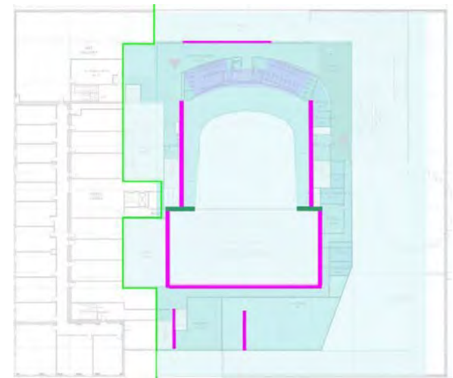
Typical Level Bracing Wall Layout
