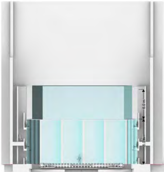
FIGURE 2: SOUND PROPAGATION - COLOURED DOTS REPRESENT SOUND PARTICLES REFLECTED FROM THE SUSPENDED CEILING REFLECTORS. THEIR GEOMETRY AND LOCATIONS ARE OPTIMISED TO PROVIDE UNIFORM SOUND DISTRIBUTION ACROSS THE STAGE.
